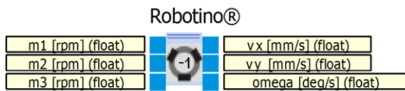
Figure 9. Functional block Omnidrive (inverse)
