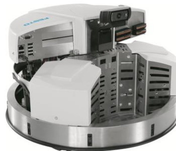
Figure 1. Mobile robot system Robotino®
